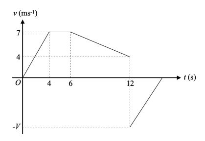
At t=0, particle P is released from rest at a point A on an inclined plane with variable magnitude of friction. The diagram shows the velocity-time graph for the motion of P. The particle passes through B at t=4, and moves from B to C with constant velocity, passing through C at t=6. The particle P has mass 0.2 kg and the frictional force acting on P between B and C has magnitude 0.4 N.
