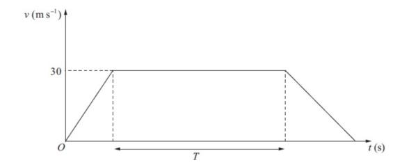
The velocity-time graph above represents the journey of a train P travelling along a straight horizontal track between two stations which are 1.5 km apart. The train P leaves the first station, accelerating uniformly from rest for 300 m until it reaches a speed of 30 ms<sup>-1</sup>. The train then maintains this speed for T seconds before decelerating uniformly at 1.25 ms<sup>-2</sup>, coming to rest at the next station.
