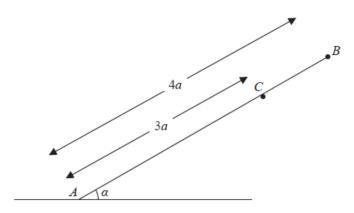
A uniform rod AB has length 4a and weight W. A particle of weight kW, k < 1, is attached to the rod at B. The rod rests in equilibrium against a fixed smooth peg. The end A of the rod is on rough horizontal ground. It is given that  $\tan \alpha = \frac{1}{3}$ .
