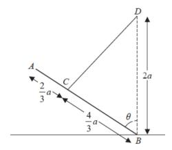
A uniform rod AB of mass m and length 2a rests with the end B on rough horizontal ground. The rod is held in equilibrium at an angle  $\theta$  to the vertical by a light inextensible string. One end of the string is attached to the rod at the point C, where  $AC = \frac{2}{3}a$ . The other end of the string is attached to the point D, which is vertically above B, where BD = 2a.
