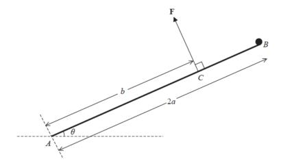
A uniform rod AB, of mass 3m and length 2a, is freely hinged at A. A particle of mass m is attached to the rod at the end B. The system is held in equilibrium by a force  $\mathbf{F}$  acting at the point C.
