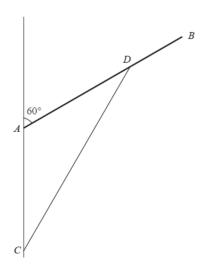
A uniform rod AB of weight W is freely hinged at end A to a vertical wall. The rod is supported in equilibrium at an angle of  $60^{\circ}$  to the wall by a light rigid strut CD. The strut is freely hinged to the rod at the point D and to the wall at the point C, which is vertically below A. The length of the rod is 4a and AC = AD = 2.5a.
