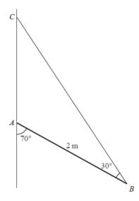
A uniform rod AB has mass 6 kg and length 2 m. The end A of the rod rests against a rough vertical wall. The rod is held in limiting equilibrium by the string BC.
